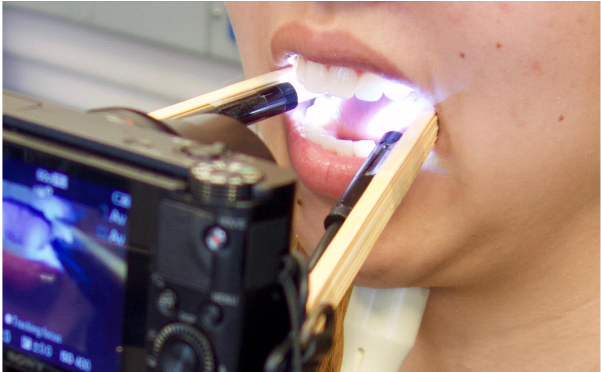
Figure 3. The experimental setup: Two bite blocks were placed in the mouth, with one on each side held by the top and bottom molars. A camera (Sony Cyber-shot DSC-RX100) was positioned directly in front of the mouth, and was manually focused on the upper molars.
